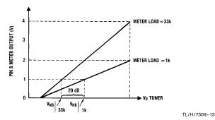
FIGURE 11. Affect of Meter Load on Narrow Band Threshold
