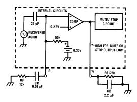
FIGURE 4. Simplified Level Mute/Stop Circuit
