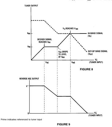
voltage, while  $V_D$  is allowed to increase.  $V_D$  will increase until it reaches the level of the wide band threshold at the tuner output. When this occurs  $V_{UD}$  is no longer needed to keep  $V_o > V_{WB}$  as  $V_D$  takes over the job. Thus  $V_{UD}$  will drop as the amount of AGC increases, while  $V_D$  is held constant by the AGC.
