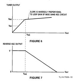
In *Figure 7* there is no AGC output until the tuner output equals the wide band threshold. At this point both SW2 and SW1 are closed and the AGC holds the tuner output in *Figure 6* relatively constant.
